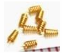
Torsion Spring Wire Dia : 0.15 mm Outer Dia : 0.8/1.05 mm Length : 1.77 mm Treatment : Gold Plated
