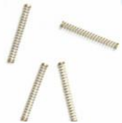
Compression Spring Wire Dia : 0.09mm Outer Dia : 0.8 mm Length : 6.2 mm
