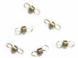
Torsion Spring Wire Dia : 0.15 mm Outer Dia : 1.0 mm Length : 2.8 mm Treatment : Gold Plated
