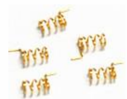
Torsion Spring Wire Dia : 0.15mm Outer Dia : 1.37 mm Length : 2.6 mm Treatment : Gold Plated
